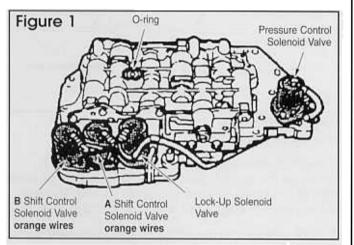
4. Remove valve body. The manual valve can come out – be careful not to drop it.
